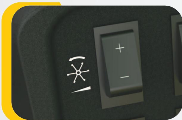
Electrically Operated Header Reel Speed Adjustment
